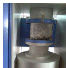
Figure Compressive strength test
