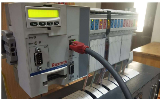
Figure 5: Indra logic kit four PLC
