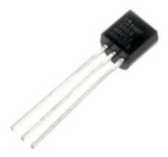
Temperature sensor is a gadget which detects varieties in temperature crosswise over it. LM35 is a fundamental temperature sensor that can be utilized for test reason. It give the readings in centigrade (degree Celsius) since its yield voltage is directly relative to temperature. It utilizes the way that as temperature expands, the voltage crosswise over diode increments at known rate (really the drop crosswise over base-producer intersection of transistor).
