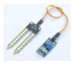
Soil dampness sensors normally allude to sensors that gauge volumetric water content. Another class of sensors measure another property of dampness in soils called water potential. These sensors are usually referred to as soil water potential sensors and include tensiometers and gypsum blocks.
