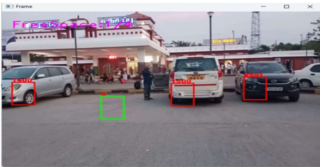
Fig. 12. Free Space Detection in Erode Junction with 1 free space
