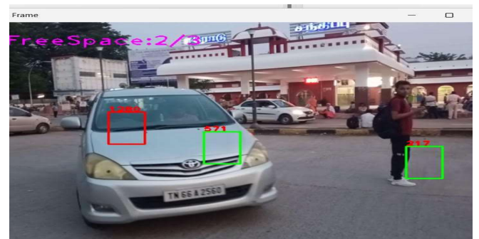
Fig. 15. Error detection due to dim light and presence of people
