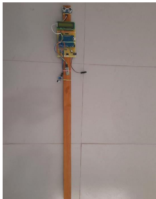
Figure 5: Smart Stick for Blind Persons
