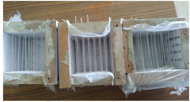
Fig. 2. Weaving of optical fibers
