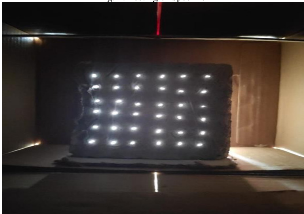
Fig. 5. Sunlight passing through the mortar cubes during daytime.
