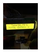
The number of people entering will be detected using the Entry Counter and the IR Sensor and the total entries will be displayed on LCD Screen.
