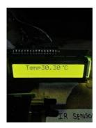
The System will detect the temperature when the user touches the LM 35 temperature sensor and will display the value of the Temperature on the LCD Screen.
