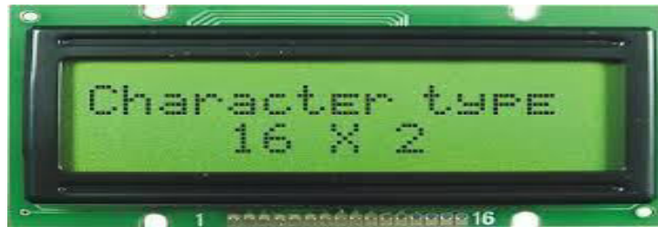
Figure 6 : 16x2 LCD display
