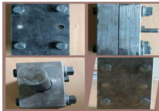
Fig.3.1:- Die Set for composites
