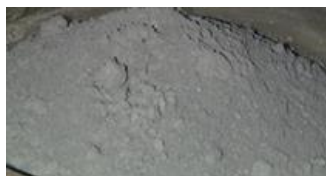
Fig.2.1: - 6061 Aluminum nano powder
